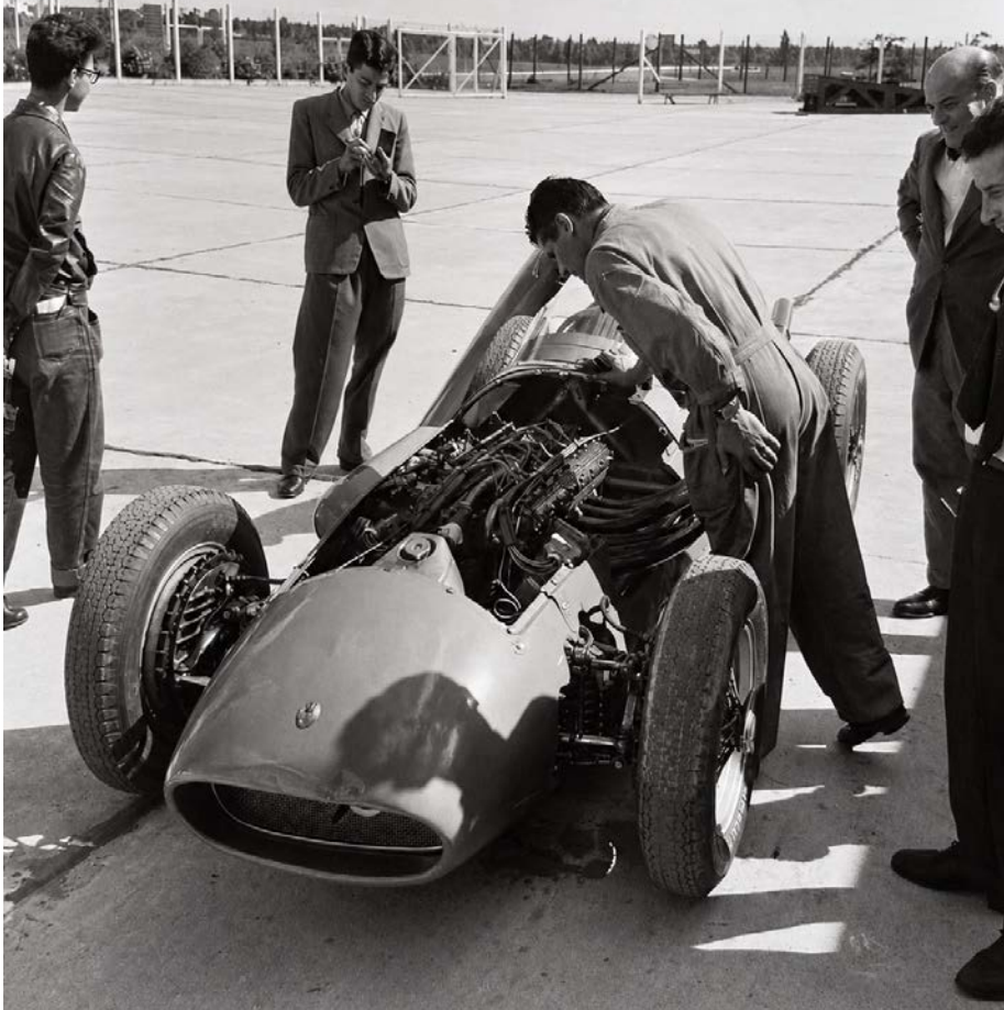
A mechanic checks #2515 to prepare it for scrutineering in Buenos Aires before the 1956 Argentine GP. The small damage on the upper front lip came during practice and was repaired for race. (Alejo Perez Monsalvo Collection)
