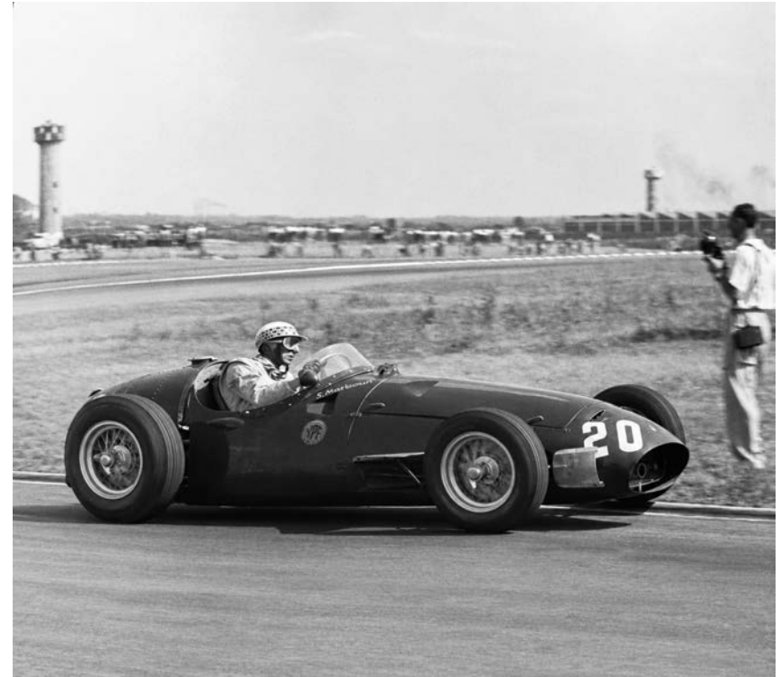
The first outing of #2515 was at the Argentine GP in January 1955. The car was in the hands of Italian driver Sergio Mantovani. Note the additional air intakes just in front of the engine bonnet and the unpainted panel that had been mounted on both sides of the front of the car. (Klemantaski Collection)
